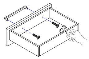
Attach handle in front of drawers, on the drilling hole position by using screwdriver to tighten bolts up.
