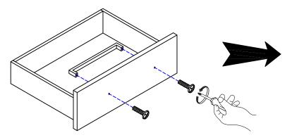
Take out handle from drawer, use screwdriver removing the bolts.
